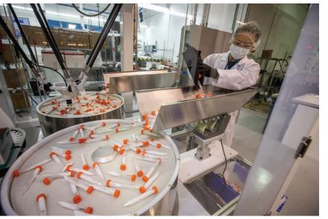
Left, "Rosie the Robot" works in the Sample Prep area, feeding empty tubes onto machines, filling them with media, then capping them. The finished products are sent over to a spider-like robot that quickly and carefully packs them into boxes, ready for customers.
