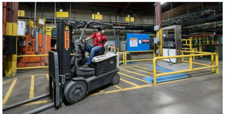
**Innovation at our Distribution Centres:** We are doing our part to bring clean and sustainable technology to communities in which we operate. At our distribution centres in Brampton and Caledon, Ontario we produce hydrogen via electrolysis to power our forklifts and other material handling equipment. Replacing the lead-acid batteries that power heavy equipment with hydrogen fuel cells significantly improves productivity levels, reduces operational costs and reduces greenhouse gas emissions.
