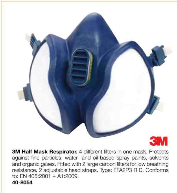
**3M Half Mask Respirator.** 4 different filters in one mask. Protects against fine particles, water- and oil-based spray paints, solvents and organic gases. Fitted with 2 large carbon filters for low breathing resistance. 2 adjustable head straps. Type: FFA2P3 R D. Conforms to: EN 405:2001 + A1:2009.
