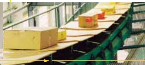
The parcels are sorted automatically by destination area ...
