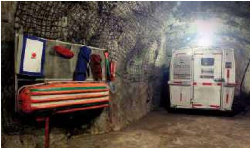
Mine rescue chamber underground at El Cubo
