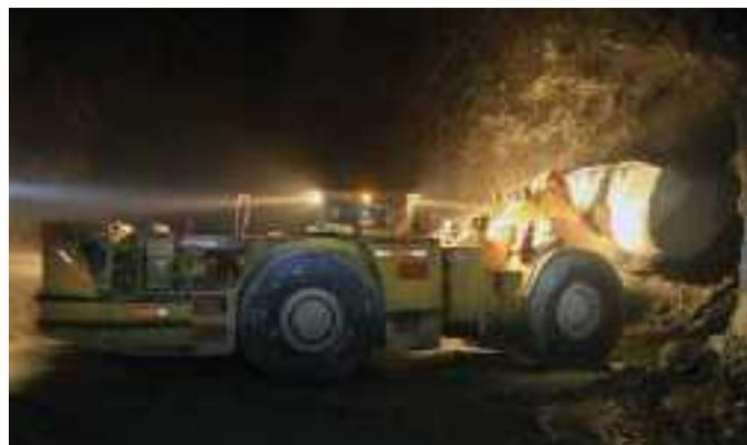
A scoop tram loading ore at Bolañitos
