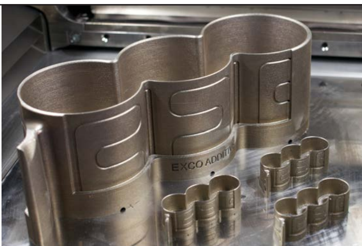
Conformal cooling channel in a 3D-printed water jacket
