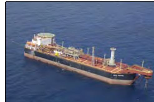
Anoa Natuna Floating Production Storage and Offloading (FPSO) vessel, Indonesia
