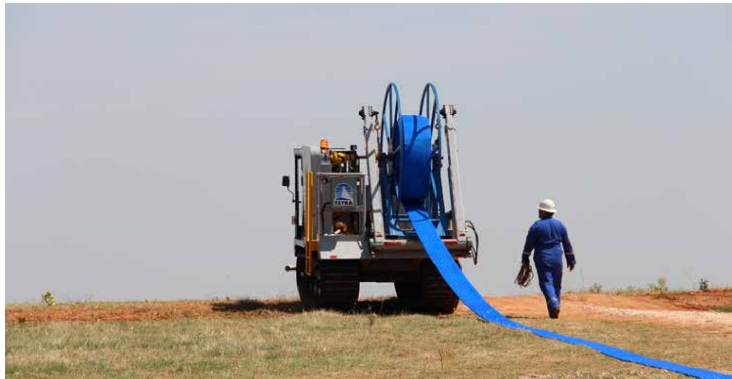
TETRA Steel™ transfer technology is the industry's only double-jacketed, UV-resistant, and quickly deployable hose.
