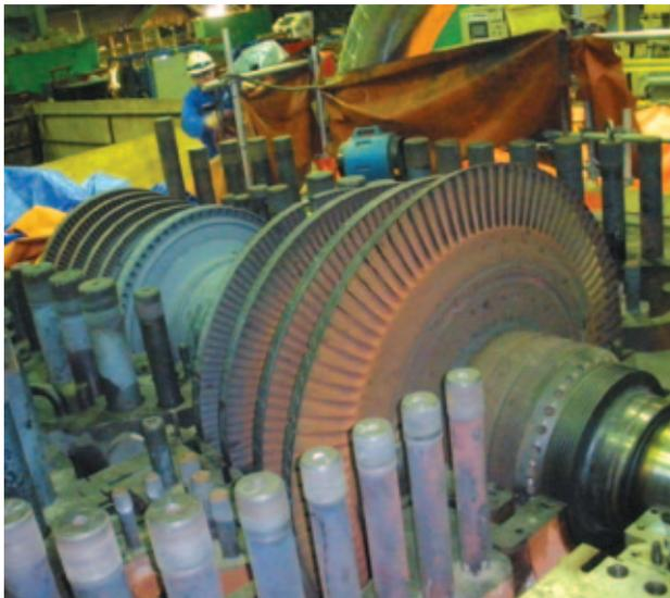
The turbine rotor during the Keephills uprates. The uprates were completed as part of a large-scale maintenance outage involving a total of 95 days, more than 900,000 work hours and 670 people on-site during peak execution across both units.
