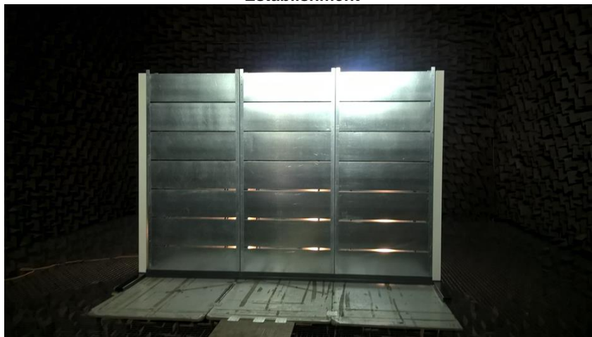
Figure 5 – Demonstration of the Sonobex system in an anechoic chamber at the British Research Establishment
