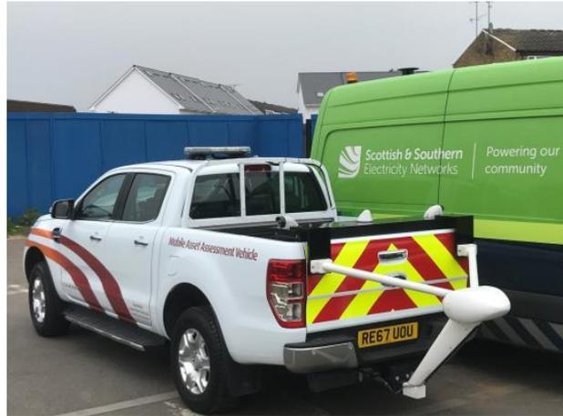
Figure 23 – UK Power Networks' MAAV next to an SSEN van while being tested by SSEN
