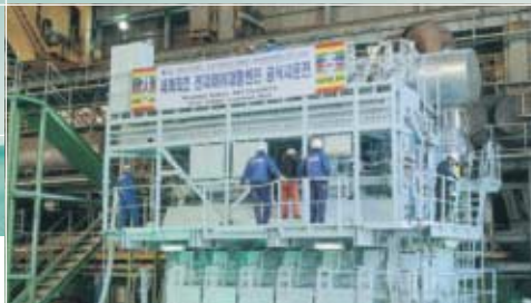
The first Sulzer RT-flex (Common Rail) engine completing its official shop test. This 6RT-flex58T-B engine develops 12,750 kW.
